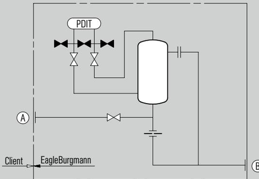
**P&ID for LSA6000-A4 Leakage collection system**
