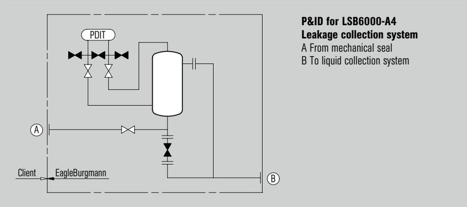
**P&ID for LSB6000-A4 Leakage collection system**
