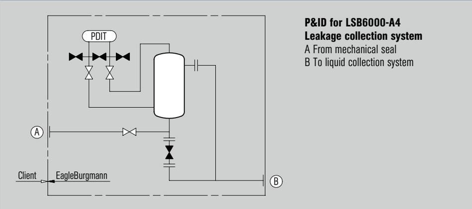
**P&ID for LSB6000-A4 Leakage collection system**
