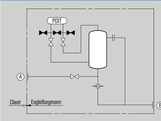
**P&ID for LSA6000-A4 Leakage collection system**
