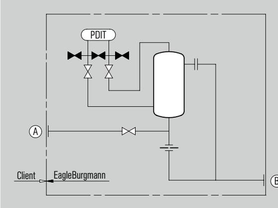
**P&ID for LSA6000-A4 Leakage collection system**
